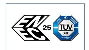
The European Norms Electrical Certification (ENEC) mark is issued for lamps and luminaires, office and multimedia equipment, as well as household appliances. The mark
